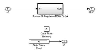
• The subsystem to be extracted contains both Data Store Write and Data Store Read blocks.
