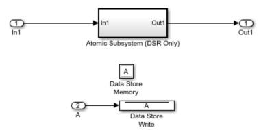
• The subsystem to be extracted contains Data Store Write blocks, but does not contain any Data Store Read blocks.
